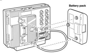
2 Insert the battery pack and slide it in the direction of the arrow.
